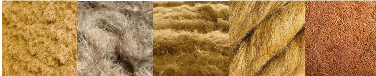
Figure 6: Natural Fibre (from left to right): Wood Fibre, Flax Fibre, Hemp Fibre, Sisal Fibre, Coconut Fibre.
