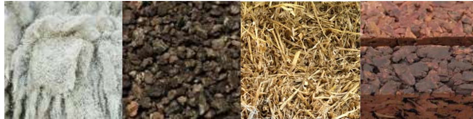
Figure 7: Natural insulation (from left to right): sheep's wool, Cork, straw, & wood bark.
