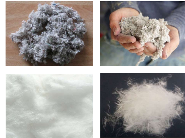
Figure 4: a) Newspaper cellulose insulation, b) PET recycled insulation, c) Polyester recycled insulation, d) Chicken feathers insulation
