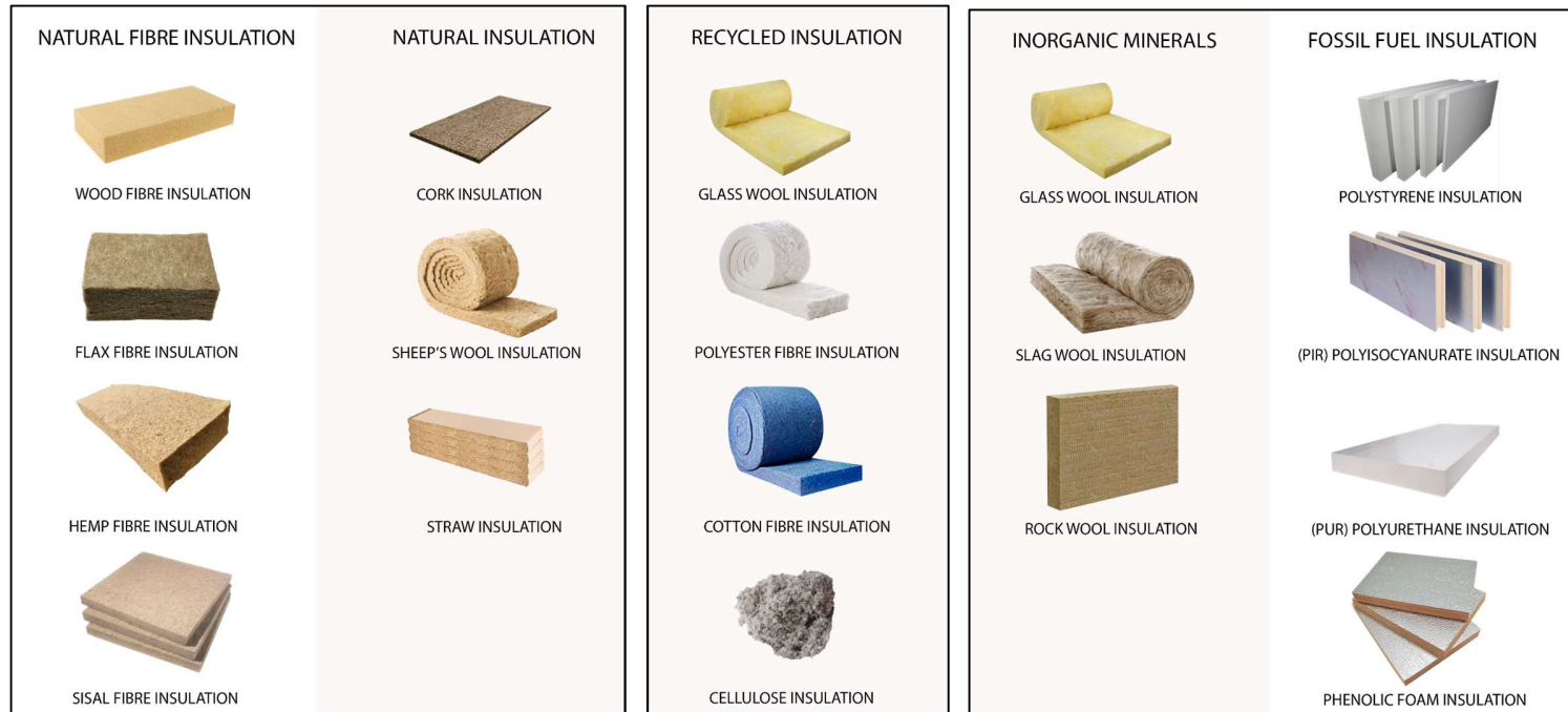
Figure 5: Building insulation example materials
