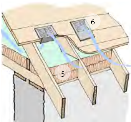
Eaves filled with insulation, roof space ventilated by fitting 'slate vents' through sarking
