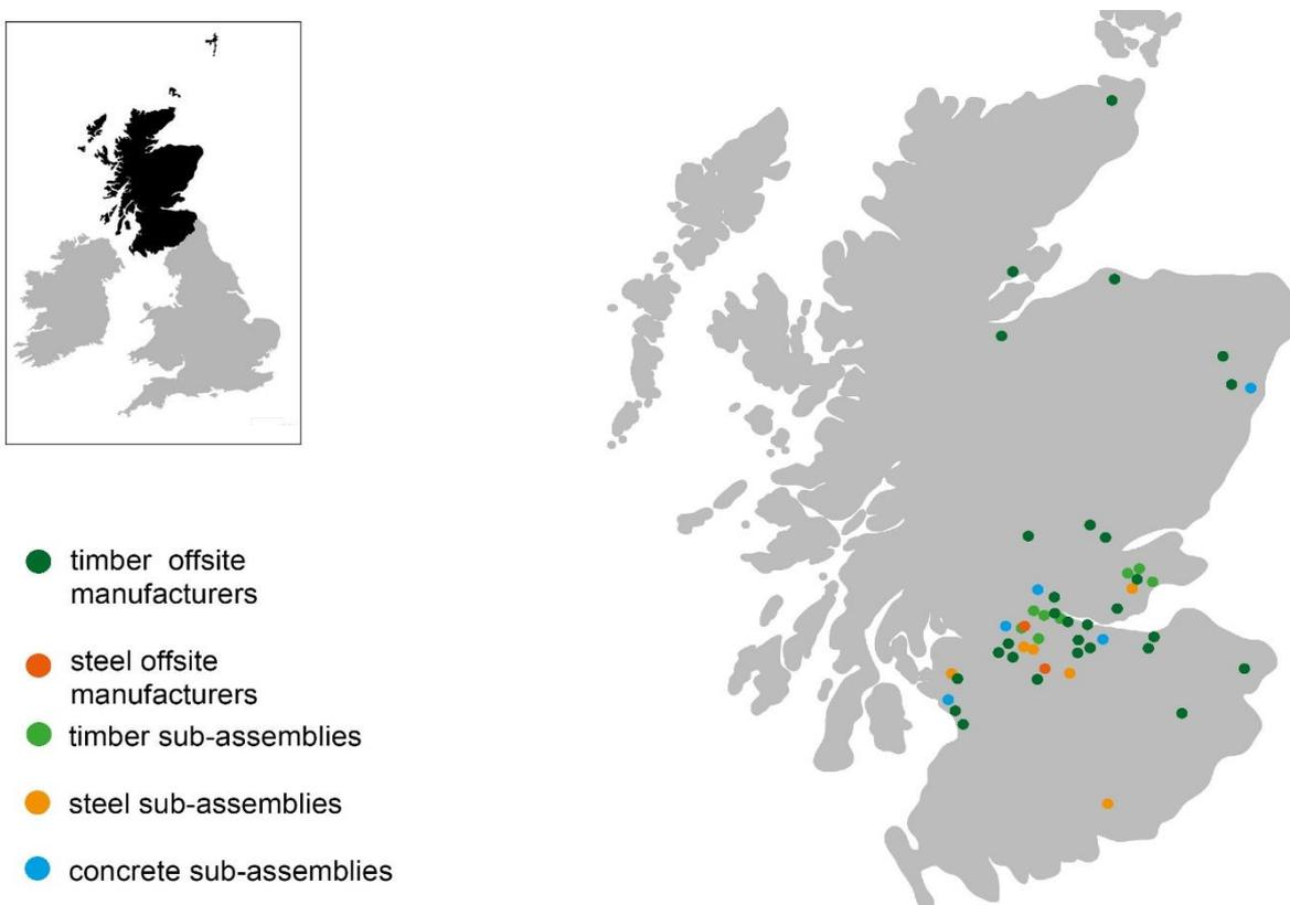
Figure 7 – Map of the Offsite manufacturers and sub-assemblies potential suppliers in Scotland identified for the study. Access to interactive online map: <http://bit.ly/companiesmap>
