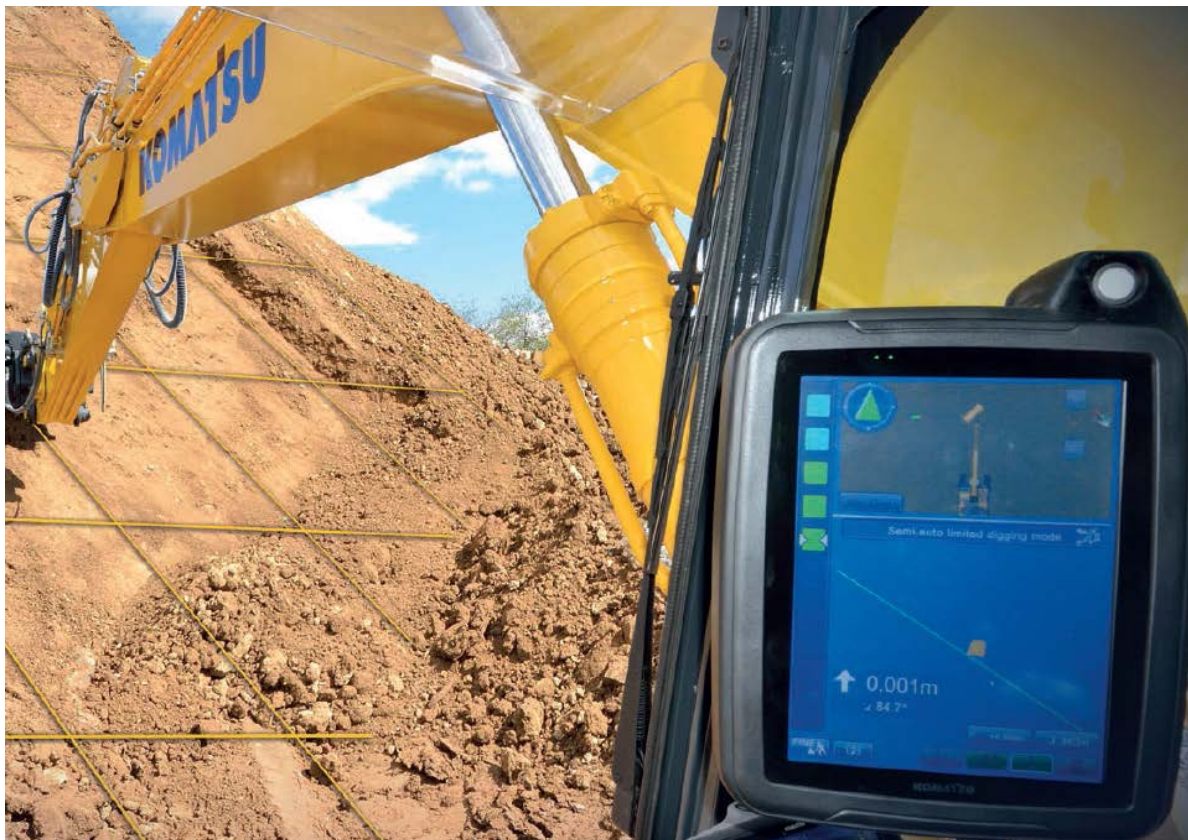
Figure 5: Intelligent Machine Control (Source: Komatsu )
